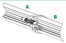
Push A and B sections together, sliding prong through location slot.
