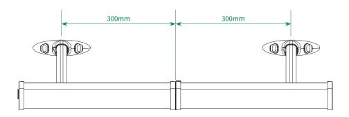
Preparation:- For best results, please fix a bracket 300mm each side of the joint.
